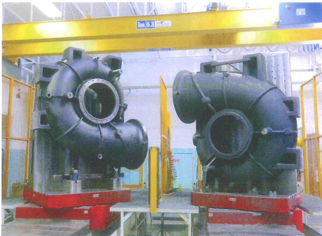
NCBK 800 670 during machining phase.
